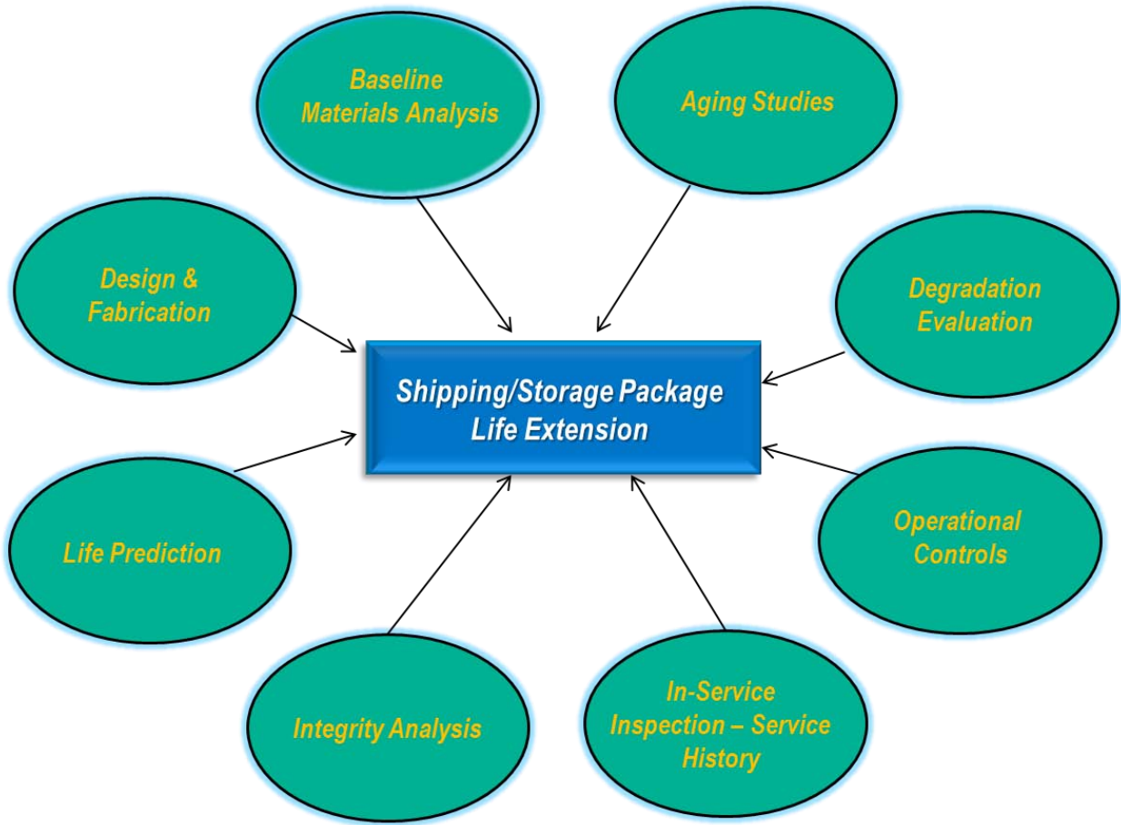
Figure 2. Schematic of general life extension program considerations for a shipping/storage package life extension program
