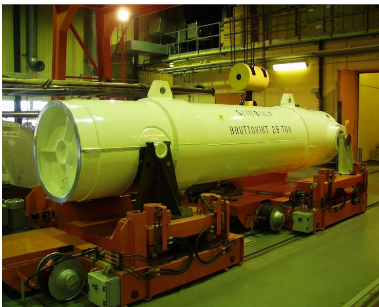
Figure 2 The Studsvik 29- tons package
