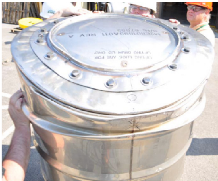
Figure 3. Damage to ES-4100 Test Unit 2 after 9-m drop test
