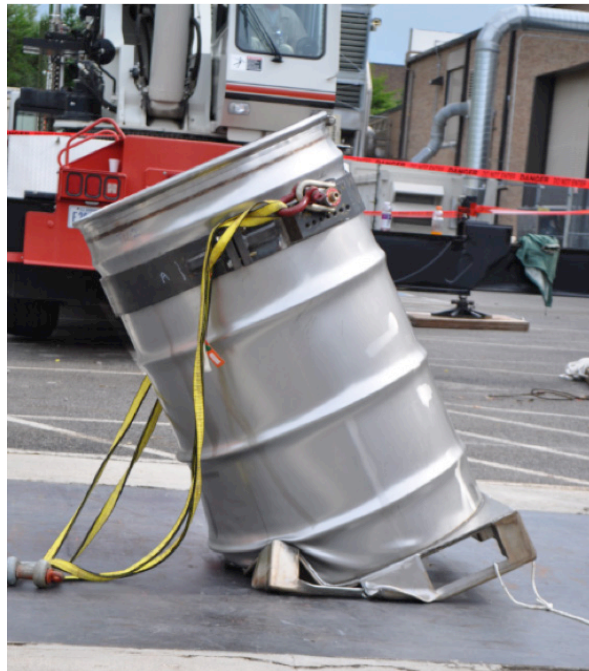
Figure 6. TRU-Shield TS-141 after CGOC on bottom drop test
