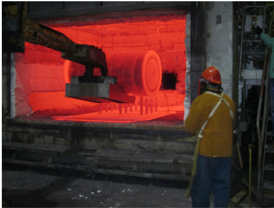
Figure 5. ES-4100 test unit being removed from furnace after furnace test
