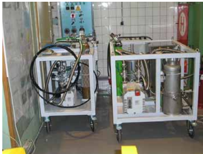
Figure 6. Drying and He-leak testing equipment sets
