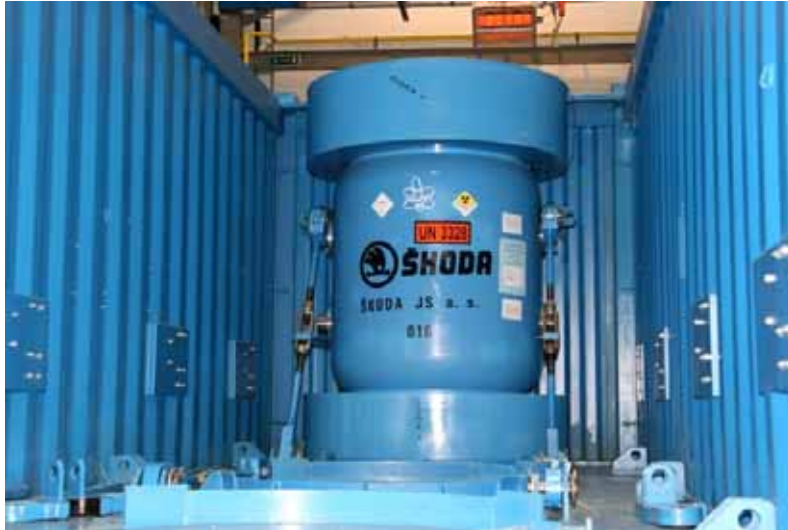
Figure 14. Cask inside the ISO container prepared for shipment
