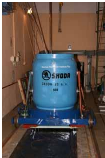
Figure 7. ŠKODA VPVR/M cask prepared for loading onto the storage pool
