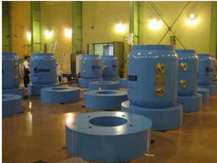
Figure 24. Casks ready for loading of SNF in Serbia
