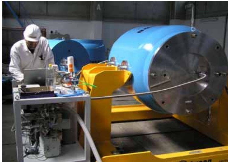
Figure 9. Cask drying, helium leak test
