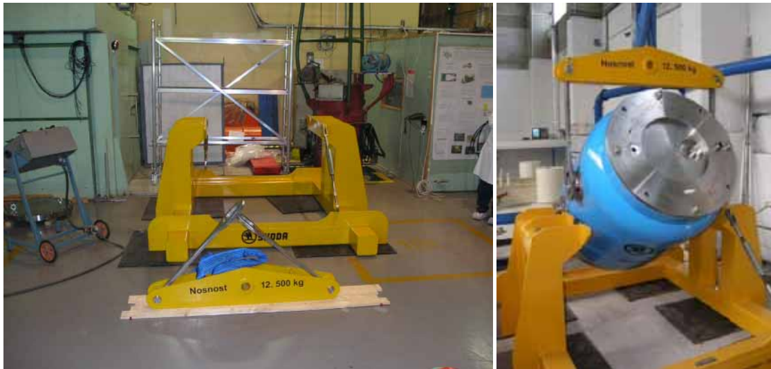
Figure 4. Auxiliary equipment sets for cask handling, in action
