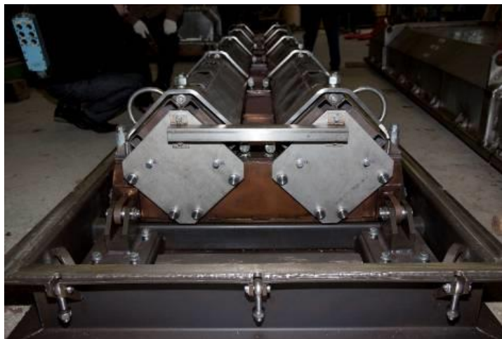
Figure 3. TUK TK-C69 containment system including a platform with cradles covered by lids
