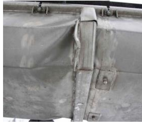
Figure 10 – Maximal damage of the packaging (TUK lid) after drop from a height of 9m by lid onto the target (in the area of ribs)
