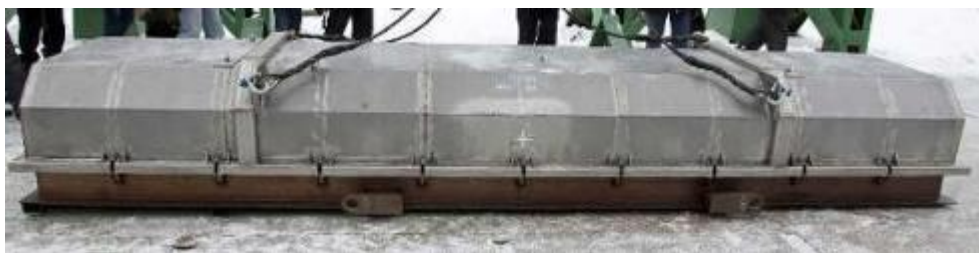
Figure 6 – The specimen state after its drop from a height of 1.2m onto the target
