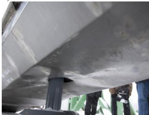
Figure 11 – The lid of the packaging specimen after its drop from a height of 1 m onto a bar
