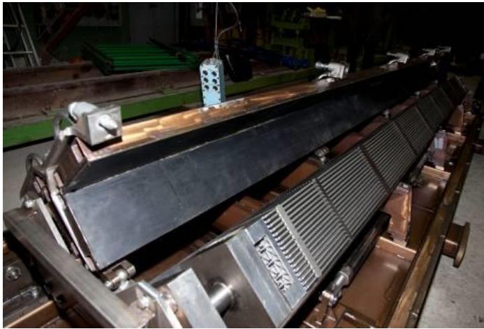
Figure 4. TUK TK-C69 containment system including a platform with cradles. One lid of the cradle is opened and a QUADRAT fuel assembly is visible.
