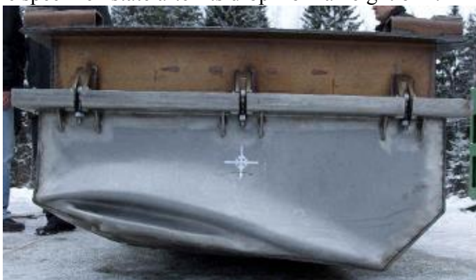
Figure 7 – The specimen state after its angular drop from a height of 9m onto the target from the side of the lid
