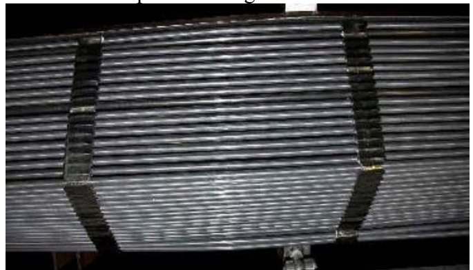
Figure 11 – The lid of the packaging specimen after its drop from a height of 1 m onto a bar
