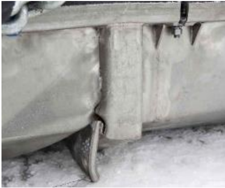
Figure 10 – Maximal damage of the packaging (TUK lid) after drop from a height of 9m by lid onto the target (in the area of ribs)
