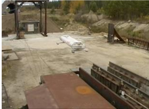
Figure 5 The TK-C5 packaging after leaving from the rail rocket track
