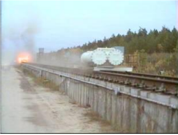
Figure 4 The TK-C5 packaging after detaching from the rocket trolley
