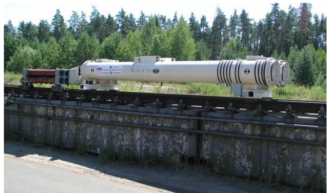
Figure 3 Rocket train with the TK-C5B packaging at the RFNC-VNIIEF rail track
