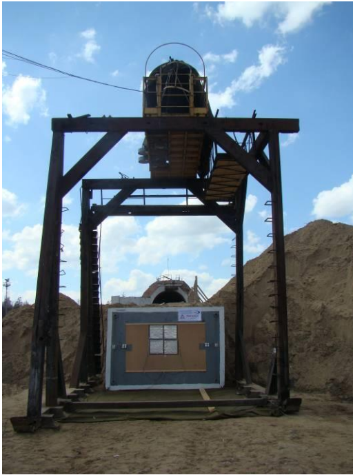
Figure 1 General view of the target used for the packaging impact testing
