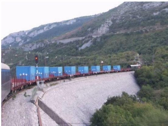
Fig. 7. Shipment of the ISO containers with the SKODA VPVR/M casks inside by rail across Slovenia (a) and their transfer onto the LYNX vessel (b)
