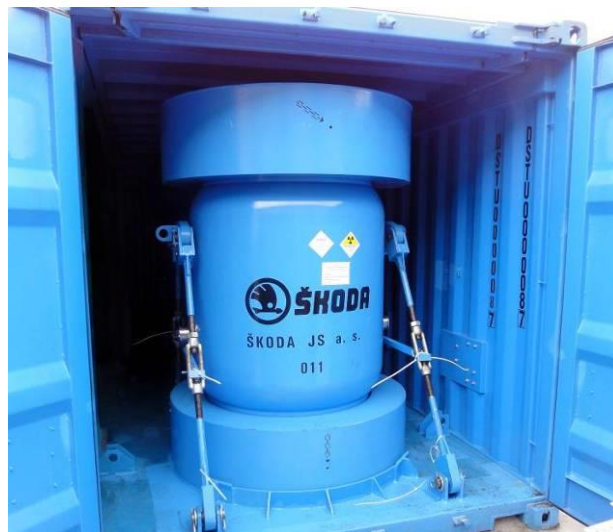
Fig. 2. The SKODA VPVR/M cask within the ISO container
