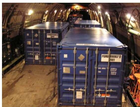
Fig. 9. The AN-124-100 Ruslan aircraft (a) and the overpacks with the TUK-19 casks inside, loaded into the cargo hold
