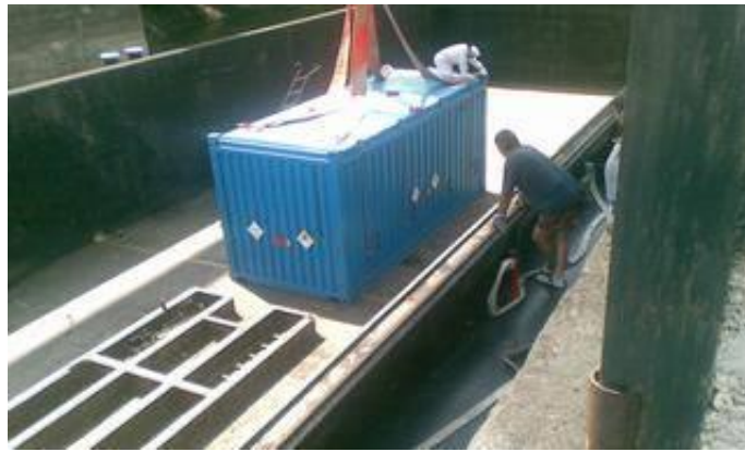
Fig. 4. Loading the ISO containers with the SKODA VPVR/M casks onto the barge of a sea-and-river type
