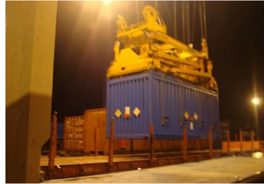
Fig. 6. Shipment of the ISO containers with the SKODA VPVR/M casks inside by road (a) and their transfer onto the rail transporters (b)
