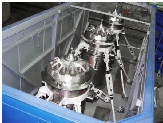
Fig. 8. An overpack made on the basis of the freight ISO container for transport of the TUK-19
