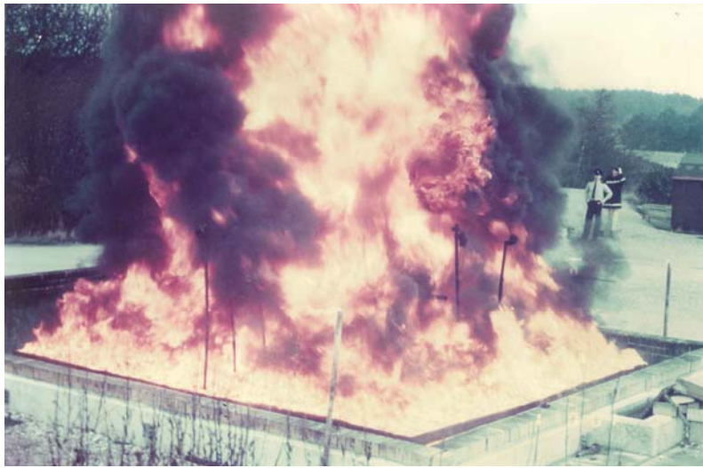
Pool fire test of wooden shock absorber
