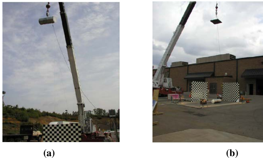
Figure 2. ES-3100 Package HAC Tests: a) Package Positioned at a 30-ft Height for Slapdown Drop, and b) Crush Plate Lifted to 30-ft Height for the Sequential Crush
