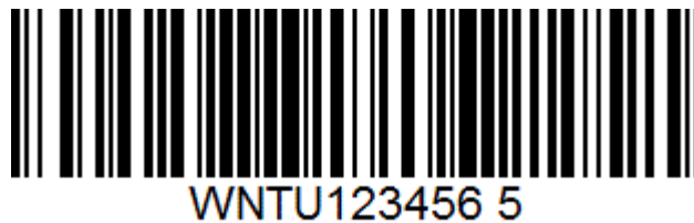
Fig. 3 Example of a Linear (1D) Barcode – Code 128
