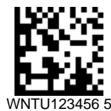
Fig. 4 Example of a Matrix (2D) Barcode – Data Matrix
