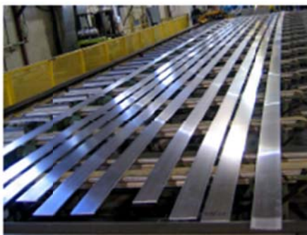
Figure 3. TN ® 24E basket boron composite material left: Profiles during manufacturing, right: B4C distribution in aluminum matrix (courtesy of AREVA TN)
