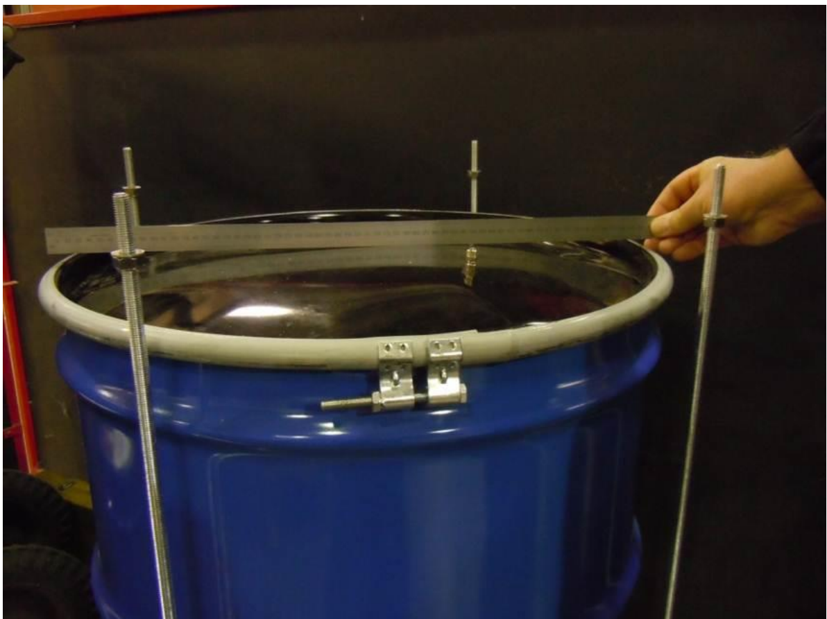
Note plastic deformation
