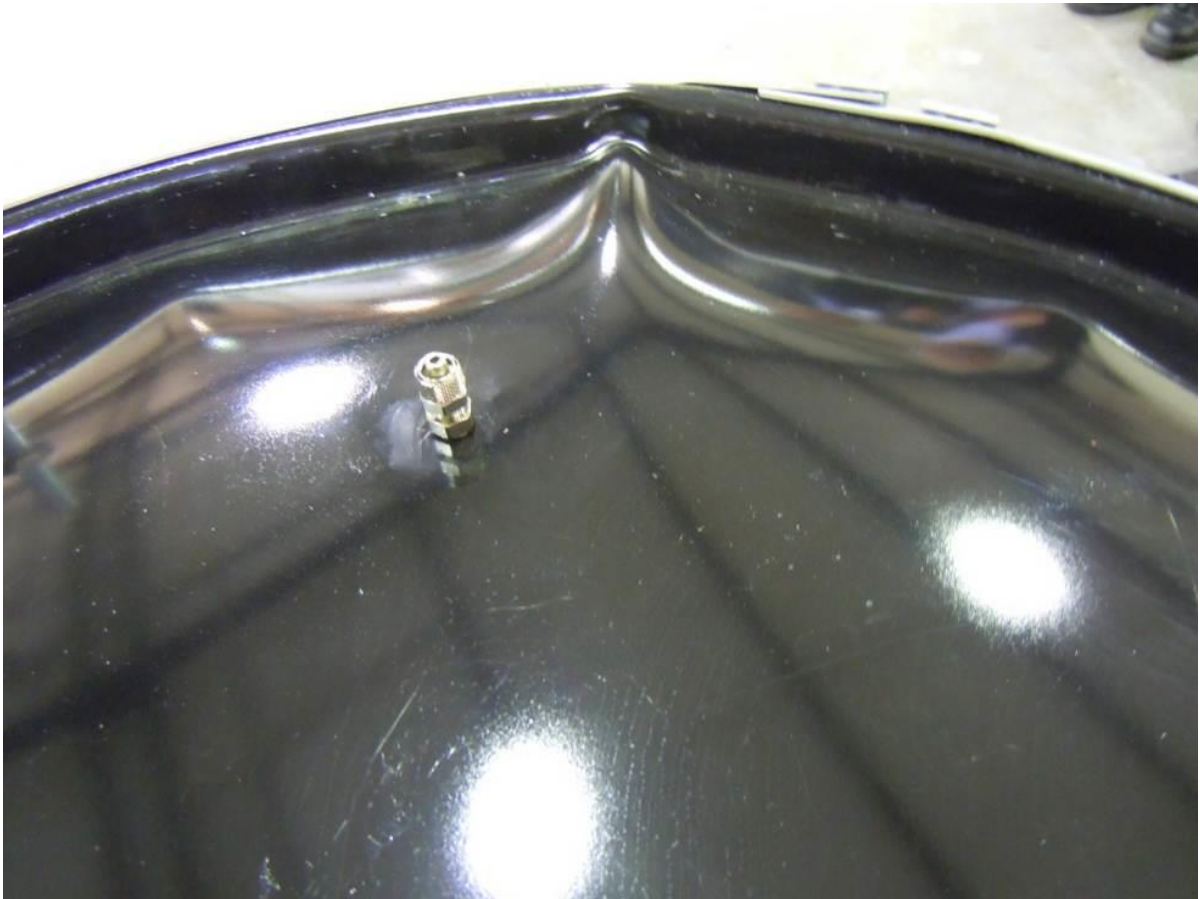
Close up of failure, note convex deformation of lid
