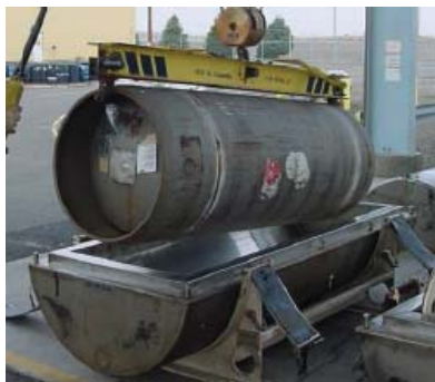
Figure 2: 30B cylinder inside the UX-30 overpack
