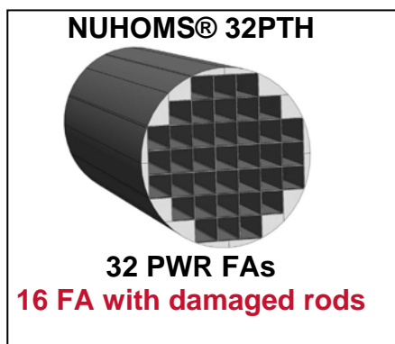
Figure 5. Example of damaged fuel rods storage license in Nuhoms® 32 PTH
