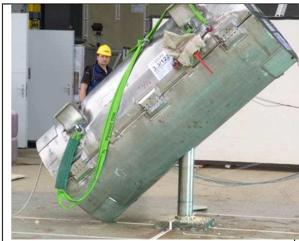
Figure 9: DN30 after bar drop
