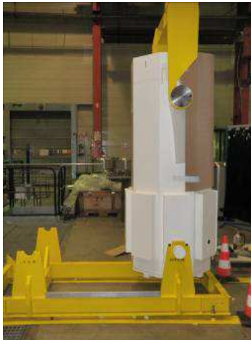
Figure 3: TN NOVA™ Mock-up for aircraft crash test
