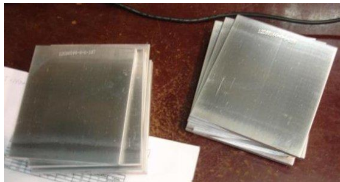
Figure 6: Marked test specimens, taken during fabrication
