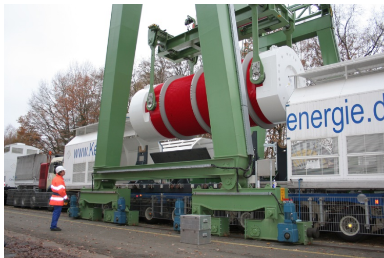
Figure 3. DPC CASTOR ® HAW28M during transportation
