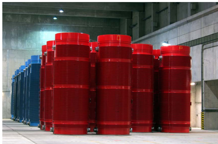
Figure 1. DPC CASTOR ® HAW28M at interim storage facility
