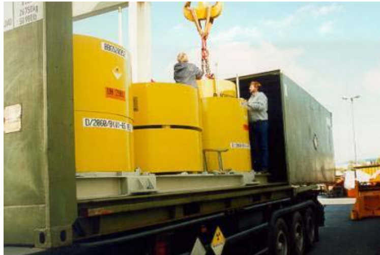
Figure 4. DPC MOSAIK ® II-15 during preparation for transportation
