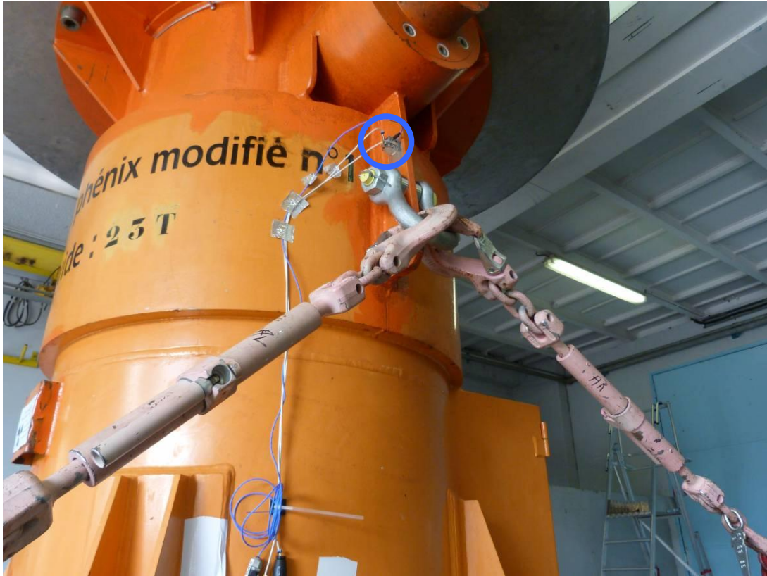
Photo 3: Accelerometer on the left side of the cask (directions X, Y and Z - ACC_EMB_G)
