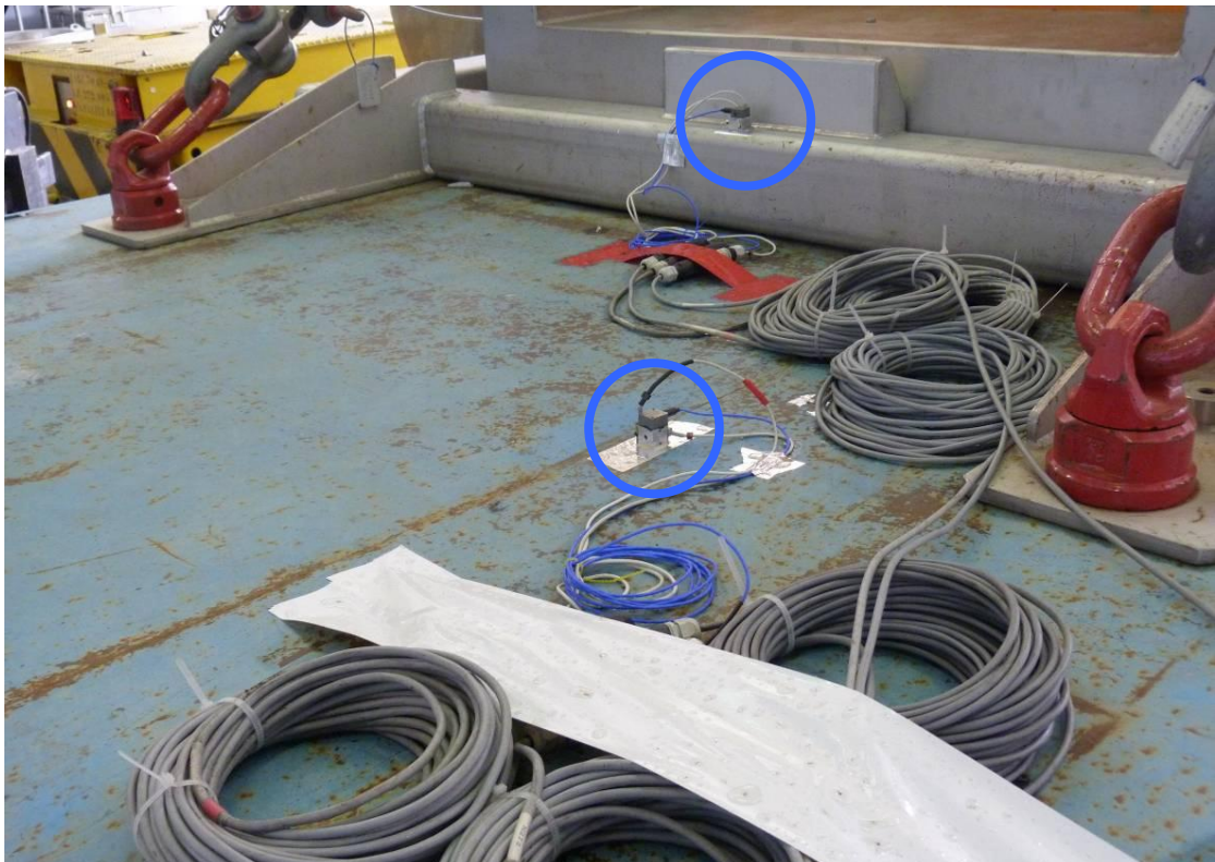
Photo 6: Accelerometer at the rear of the transport frame (directions X, Y and Z - ACC_SUP_AR) and trailer accelerometer at the rear (directions X, Y and Z - ACC_REM_AR)
