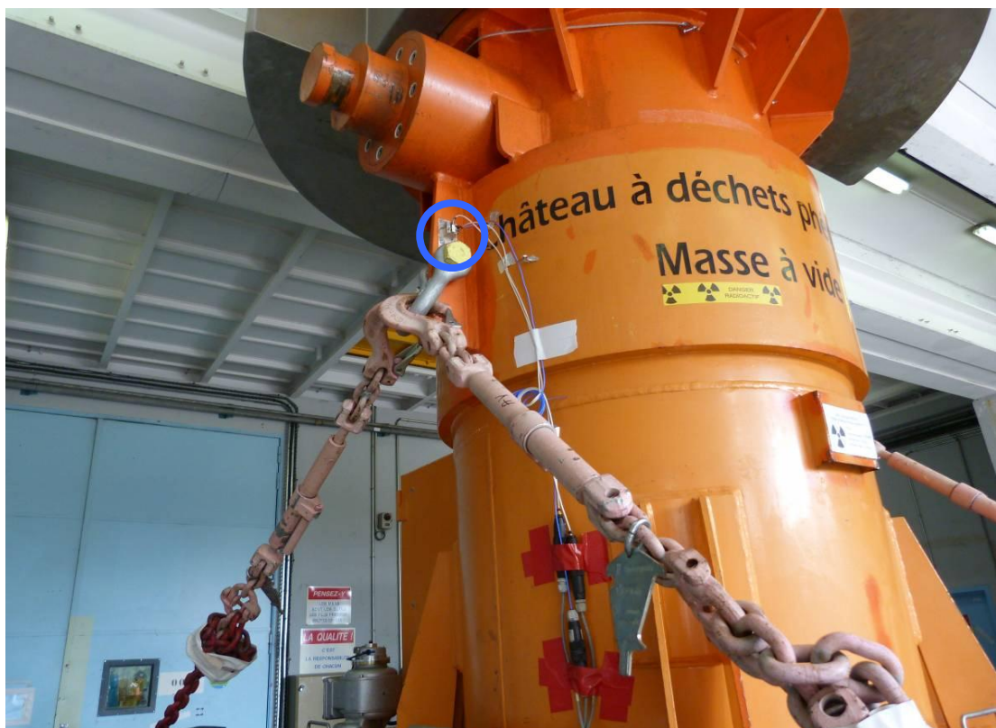
Photo 2: Accelerometer on the right side of the cask (directions X, Y and Z - ACC_EMB_D)
