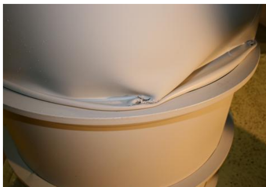
Picture 4. Mayor deformations of the outer EB3-A400/300 drum after 9 m crush test
