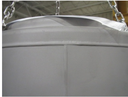
Figure 9. Containment vessel lid showing welded construction.
