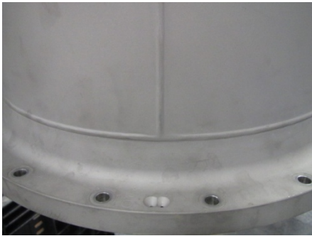
Figure 9. Containment vessel lid showing welded construction.
