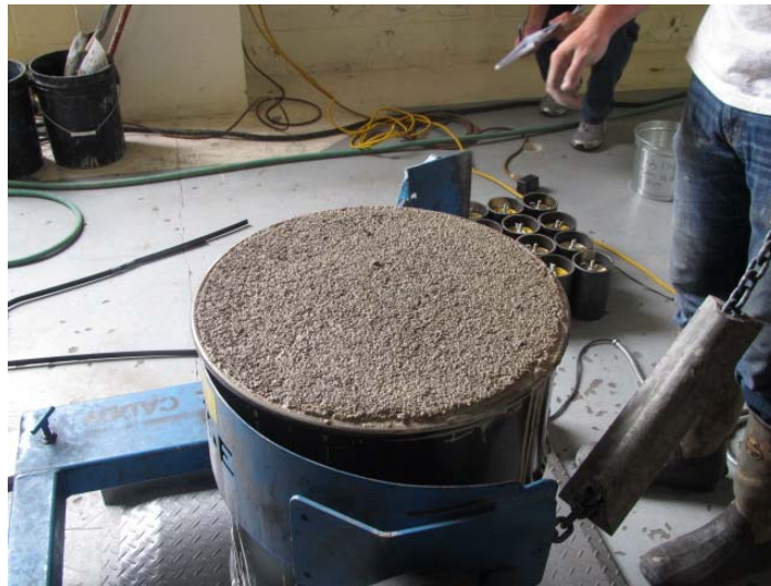
Figure 16. MD-2 after Packcrete pouring.
