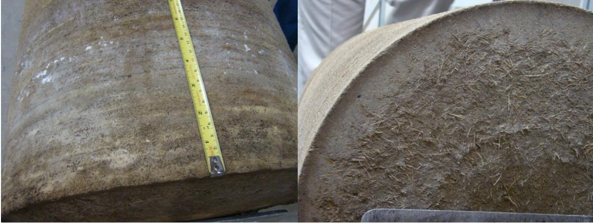
Figure 4. 9975-01818 With Excess Moisture resulting in compression and mildew
