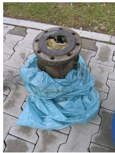
Figure 2. Incrustation from the processing of raw materials Scale: up to 310 Bq/g Ra-226
