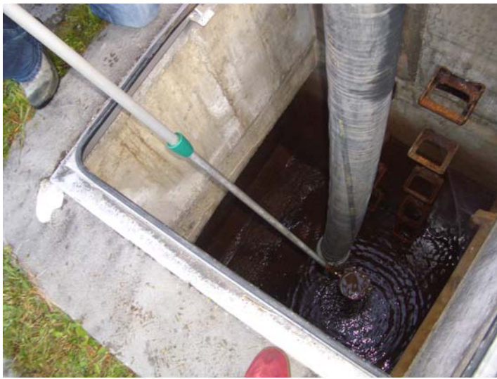
Figure 1. Filter residues from public water purification Sludge (dry): up to 60 Bq/g Ra-226
