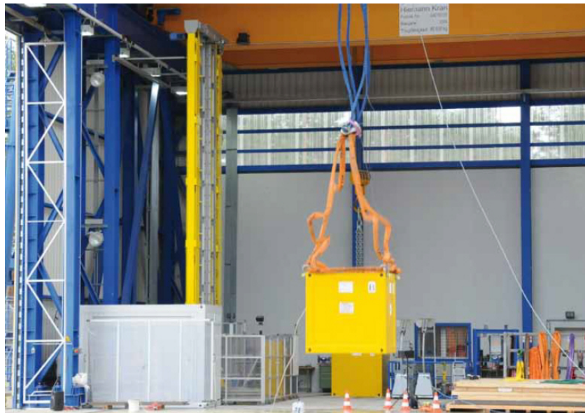
Figure 2. Packaging drop test (LLW container at BAM Test Site Technical Safety)
