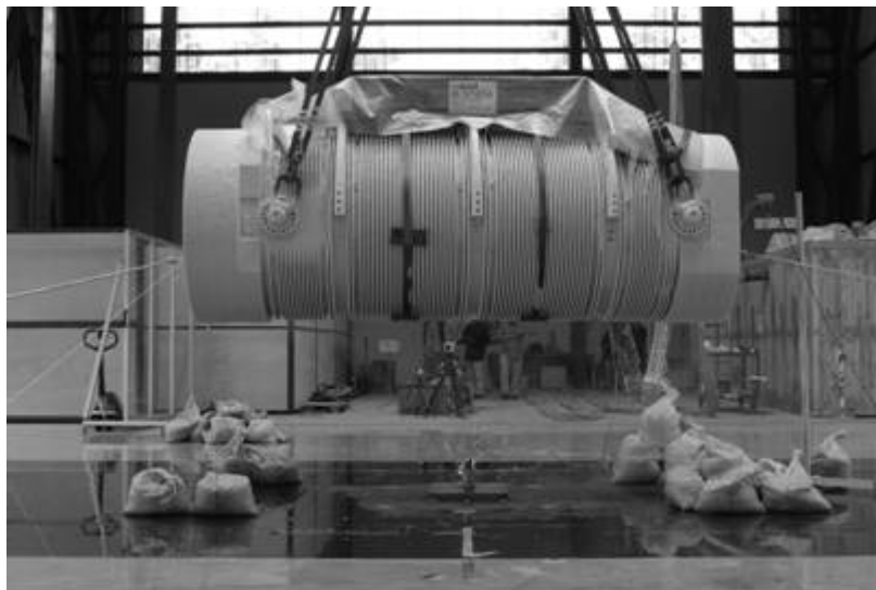
Figure 2. 1m pin drop with a half-scale drop test model
