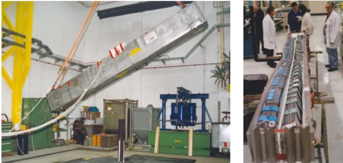
Figure 4. Testing of packages for transport of fresh fuel assemblies; 1-m puncture bar drop with ANF-10 package (left); internals of opened RA-3D package after a drop test sequence
