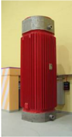
Figure 2. CASTOR ICDIORIT since 30 years in operation (Foto: Paul-Scherrer-Institute)
