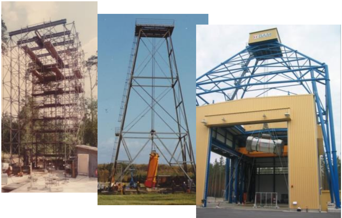
Figure 6. BAM's outdoor drop test facilities, Berlin-Grunewald (right, 1975-1980), Lehre (middle, 1978- 2005), BAM TTS (right, since 2004)
