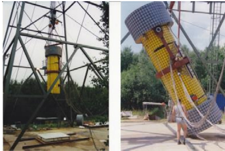
Figure 3. POLLUX cask for transport, storage and disposal of SNF; left: 5-m drop onto concrete, right: preparation for 9-m drop with lid corner onto unyielding target (BAM Lehre, 1994)
