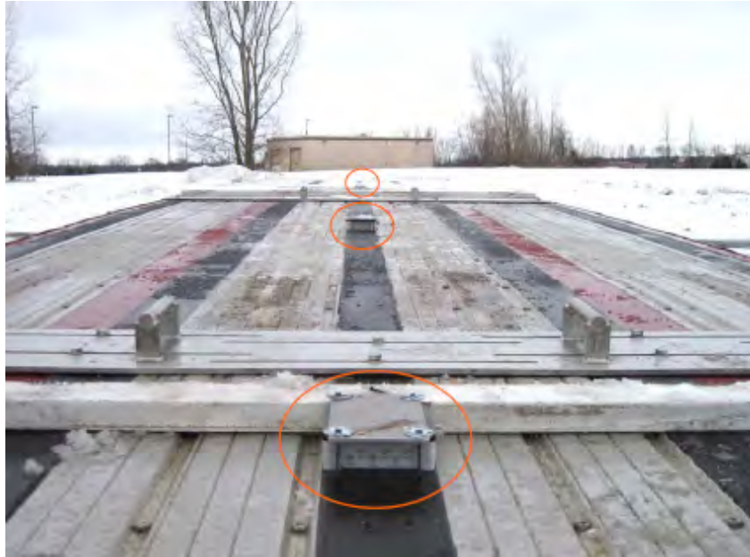
Figure 7 – Accelerometer Monitor and Recording Device on Trailer Bed
