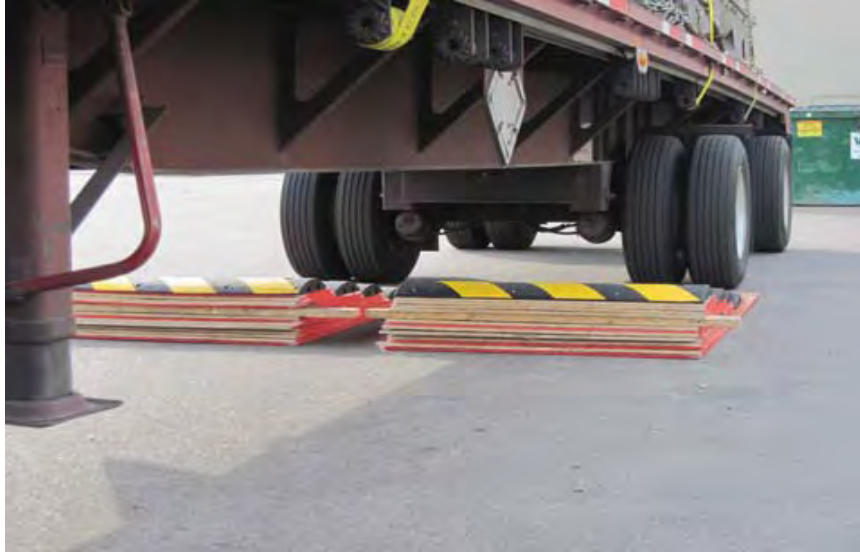
Figure 11 – Example Curb Fabricated for Shock Test
