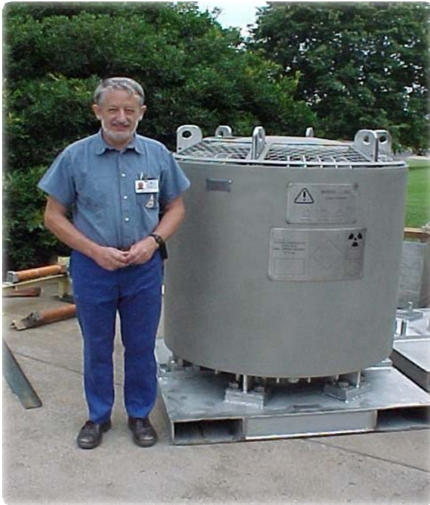
Cobalt Transport Container (250 kCi Capacity, 7Te)
