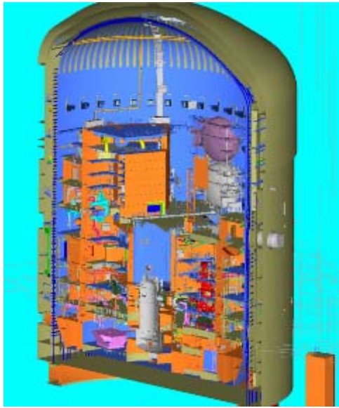
Section of the reactor building
