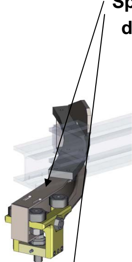
Upper Roller-& ball bearings assemblies (#2 per door)
