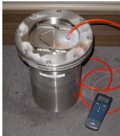
Figure 5 Showing a Type A containment undergoing soap solution testing whilst pressurised internally to 1 bar.
