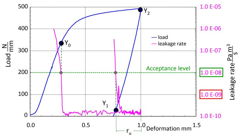
An essential parameter of a metal seal under relevant stress conditions is the useable resilience  $\mathbf{r}_{u}$  as the difference in vertical seal dimension between the assembling configuration at operating point  $\mathbf{Y}_{2}$  and point  $\mathbf{Y}_{1}$ , where the leakage rate by means of external load relieving exceeds the specified value of  $10^{-8}$  Pa·m<sup>3</sup>·s<sup>-1</sup>
