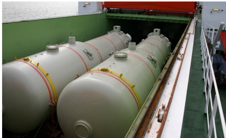
Figure 7. Steam generators (NPP Stade) inside the hold of SIGYN sea ship
