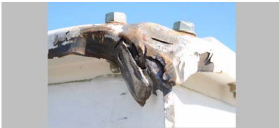
Figure 11. Deformation in waste box after CG/corner 1.2 m drop (minor deformation).
