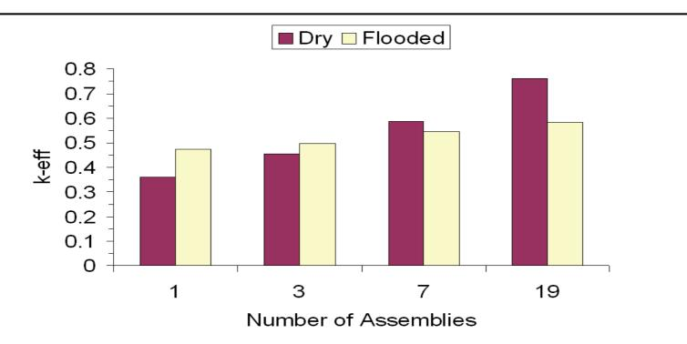
Reactivity of different numbers of ABR used fuel assemblies under dry and fully moderated conditions
