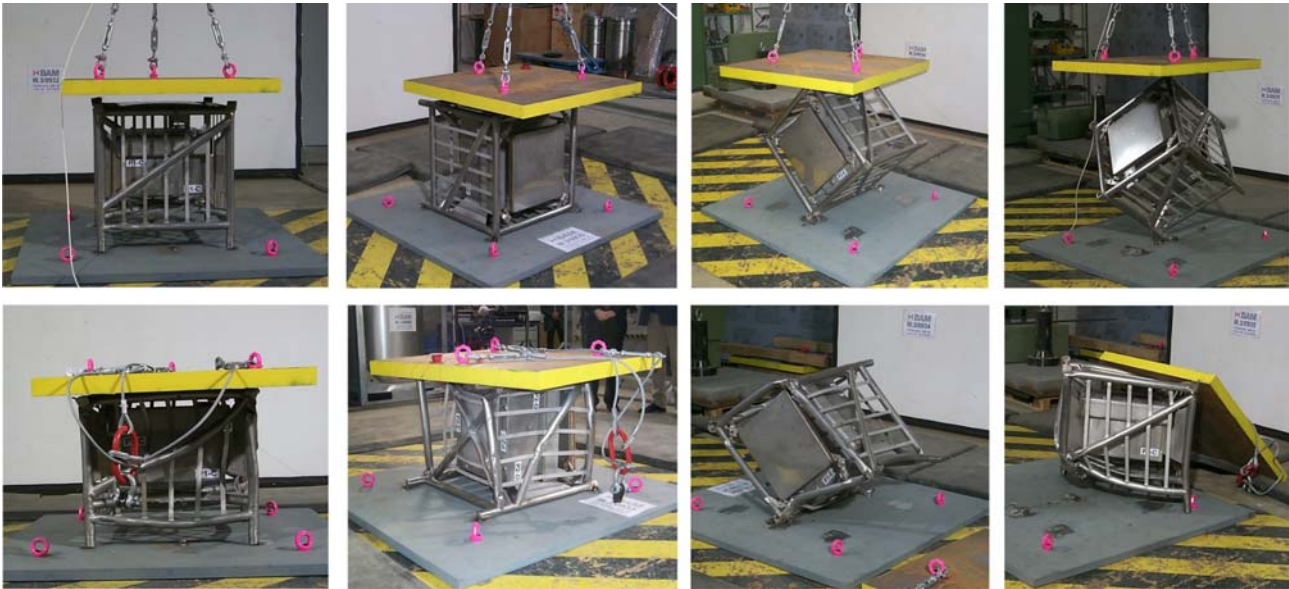
Figure 5. Dynamic crush test configurations for the ANF-50 (first line) with results after crush testing (second line).
