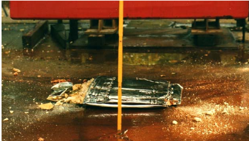
Figure 2. Crushed BAM Demonstration Package which met the IAEA requirements
