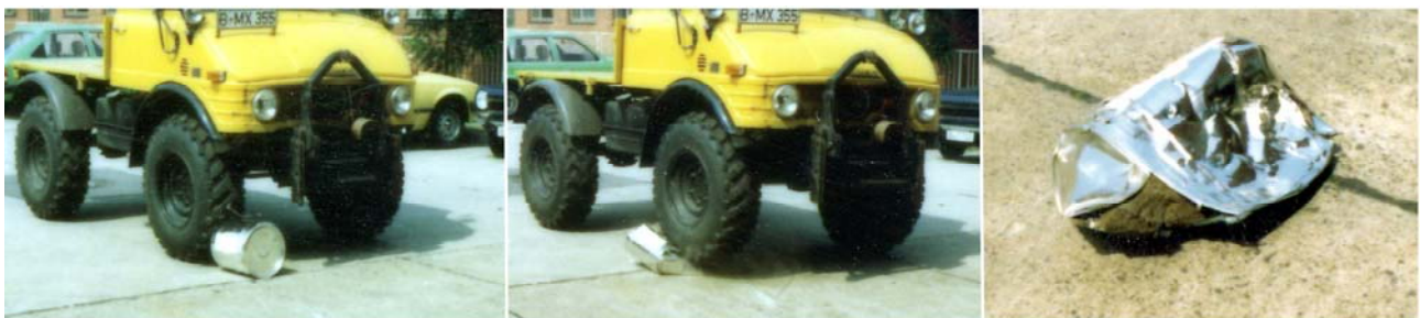
Figure 3. BAM Demonstration Package crushed by a truck run over
