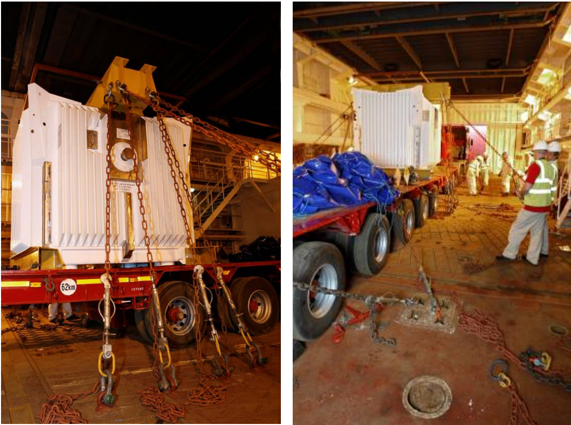
Figure 2 (left shows package tied down to ship, right shows lorry tied down to ship)
