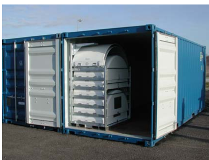
Figure 5: CTP cages secured in ISO box
