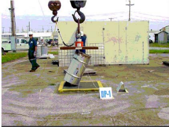
Figure 10. Crush Test of 9977 General Purpose Fissile Package (GPFPP). 6-7
