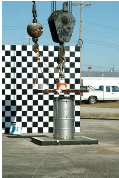
Figure 11. Rigging of the crush plate for a 9977 crush test of package in vertical orientation. 6-7
