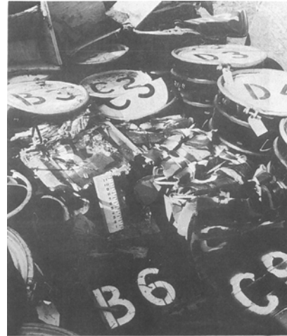
Figure 3. Effects of barrier crash on packages. Oak Ridge 20 in. Birdcage and Dow KKD-1 Packages in damaged array, prior to removal. 1966 Aberdeen Proving Ground testing. 4
