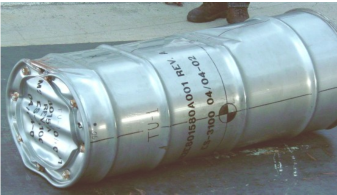
Figure 15. Damage resulting from crush test in horizontal orientation of ES-3100. (Photograph courtesy of Oak Ridge National Laboratory.)
