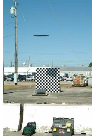
Figure 12. Crush plate falling for 9977 crush test for horizontal package orientation. 6-7
