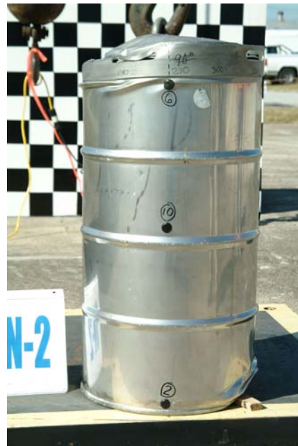
Figure 13. Damage resulting from crush test in Center of Gravity Over Corner (CGOC) orientation. 6-7
