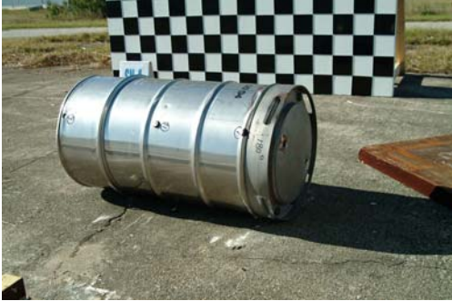
Figure 14. Damage resulting from crush test in horizontal orientation. 6-7
