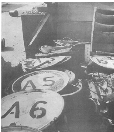
Figure 2. Effects of barrier crash on packages. Los Alamos BE1736 packages in damaged array, prior to removal. Note loss of vermiculite, drum covers and failure of locking ring. 1966 Aberdeen Proving Ground testing. 4
