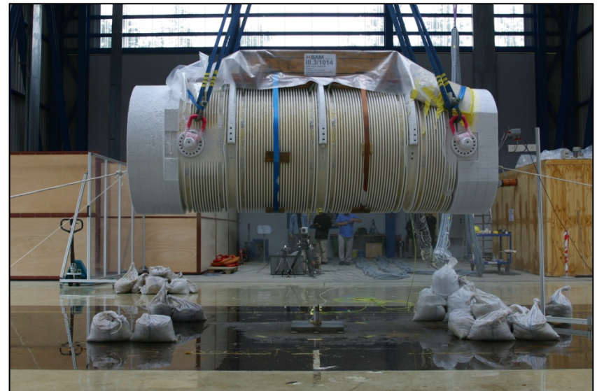
Cask before puncture drop test, cooled down to a temperature of -40^{\circ}\text{C}
