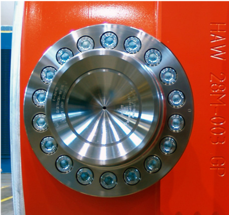
Real trunnion on a CASTOR HAW 28M (with a cap in the center)
