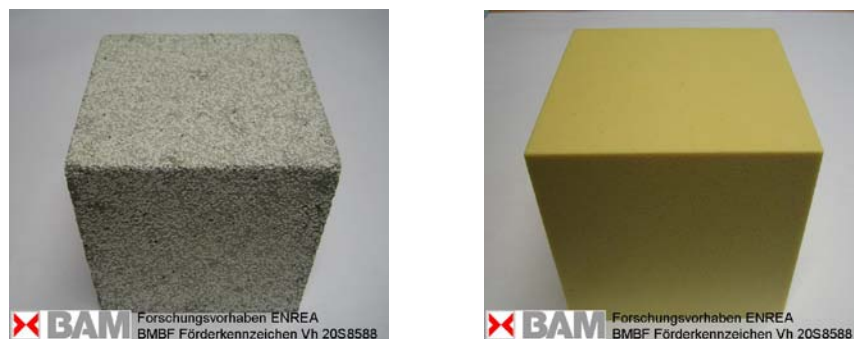
Figure 3. Specimen of damping concrete and polyurethane foam
