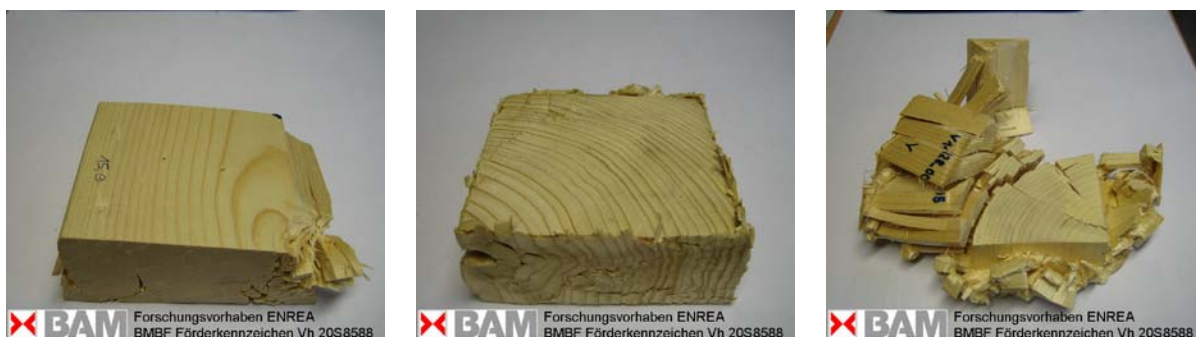
Figure 7. Wood specimen after compression
