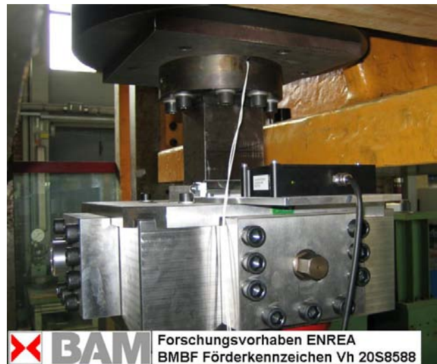
Figure 5. BAM-developed specimen holder and servo hydraulic test setup
