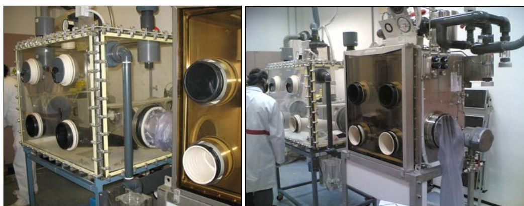
Figure 2. New glove-box system installed in PERLA for venting purposes
