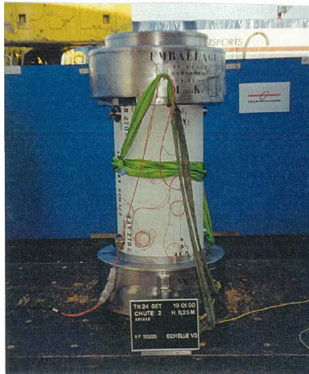
Figure 2: Vertical drop test of TN ® 24 GET scale model
