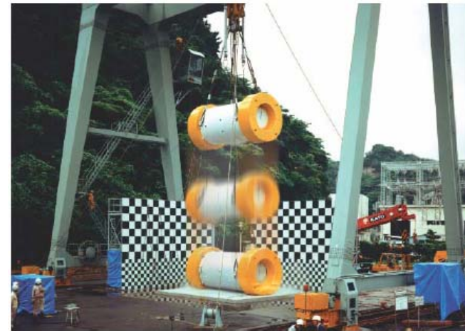
9m drop test with DCI Cask
