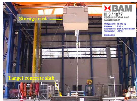
Figure 1. Storage cask at the BAM drop test facilities
