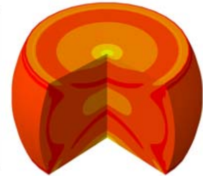
v. Mises stress from thermo-mechanical coupled calculation
