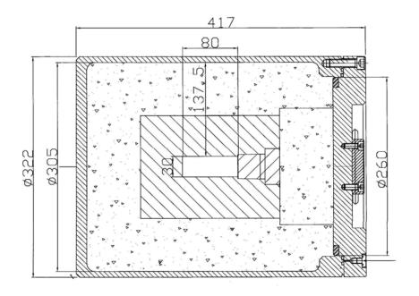
The new containment system is composed by a primary shield realized in tungsten, followed by a secondary shield of lead.
