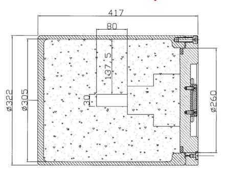
The container is totally realized in lead surrounded by a AISI 304 stainless steel liner with thickness of 17 m
