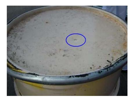
In the future we shall use the same packages as Type IP-3 for LSA-III too, so we performed the free drop test, the stacking test and the penetration test
