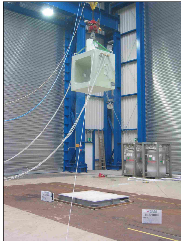
Figure 1. Drop test with the hollow section B2 from a height of 3.2 m onto the reference target
