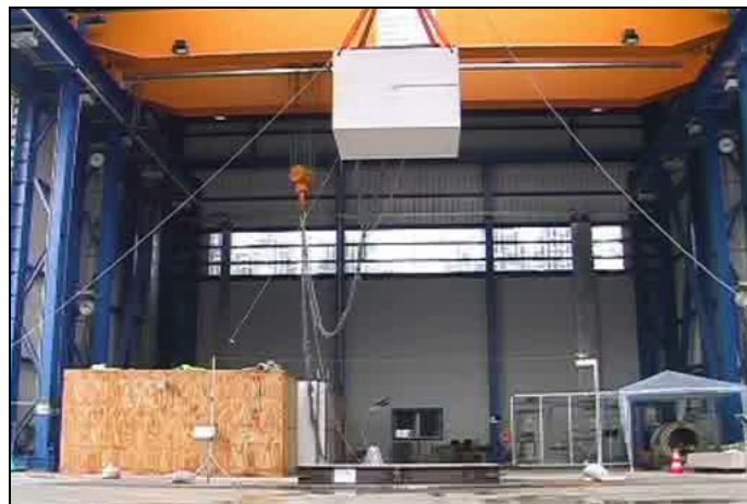
Figure 6. Drop test with container GC FORM II from a height of 5.55 m
