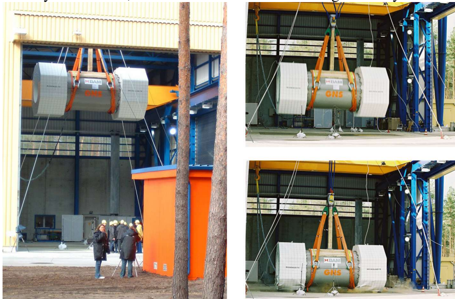
Figure 1 Drop Test with the CONSTOR® V/TC
