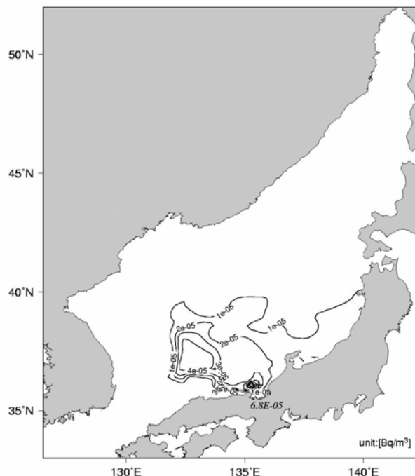
Figure 2. Horizontal distribution of total concentration of 6 radionuclides at 2 years after release from a package at the bottom of 200m depth in front of Wakasa Bay.
